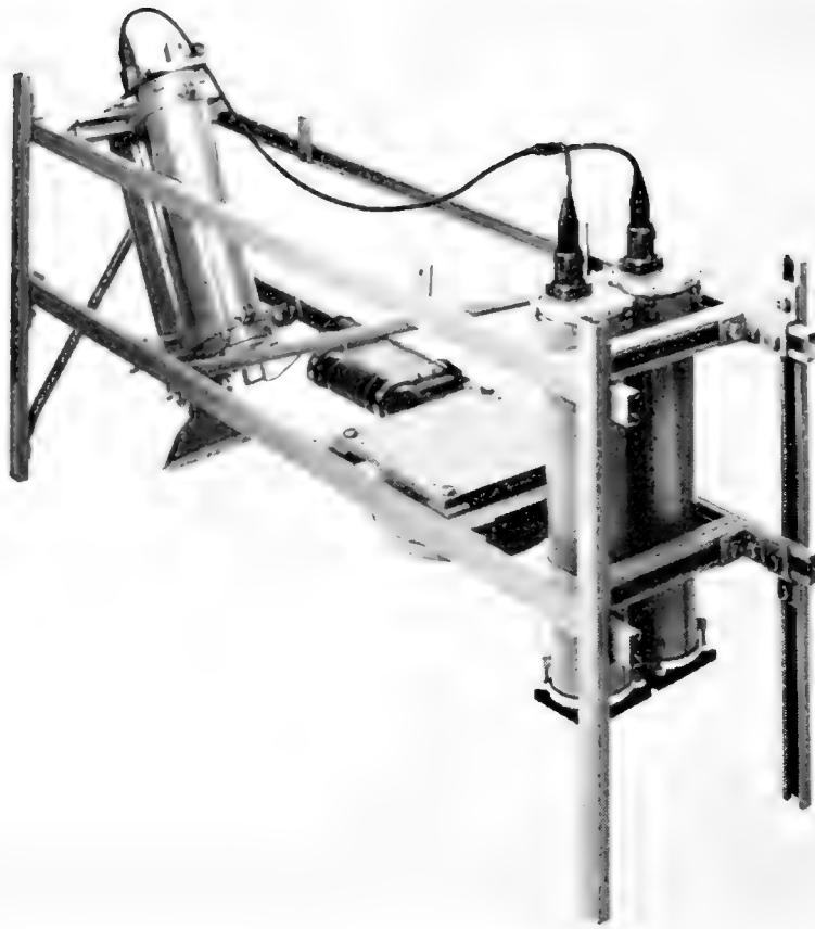
Fig. 2. A typical camera assembly for vertical stereophotography of the sea bottom. Two cameras at the right operate in synchronism with the flash lamp at the far left. Above the lamp is the sonar driver. The square flat object at the center of the framework is a 12-kc pulse sonar transducer for camera-bottom measurement.
